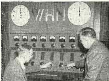
Center section of the master audio control setup being built for WHN. Equipment with six studio-control consoles and twelve audio racks will be installed in the new WHN studios at 711 Fifth Avenue, New York City. At the controls are H. J. Lavery (left) and J. F. Palmquist of the RCA broadcast audio section.
