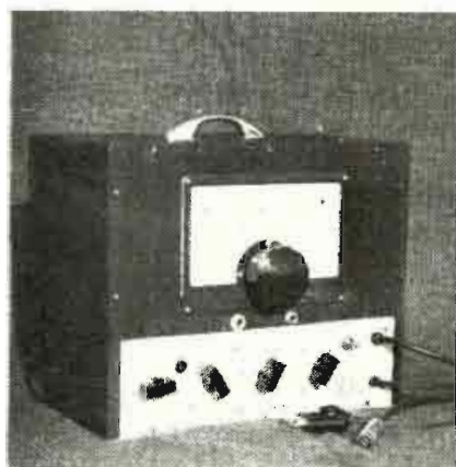
Front view of signal generator. Controls are, from left to right: Zero set variable capacitor, bandswitch with four positions, modulation with 30%, 50% and 100% points marked, r-f output 1000-ohm control with the power switch on the same shaft, and a lushi output toggle switch which can be seen above the small scale neon on indicating light.
