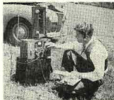
Eidson at the controls of the field-strength meter used at WIS.
